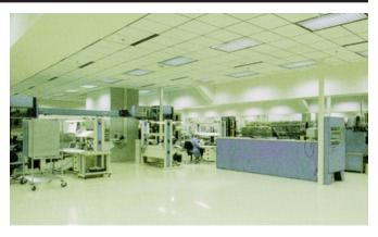
In the circuit board assembly area at Allen-Bradley, a static dissipative floor helps ensure product quality.
